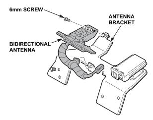
18. Plug the bidirectional antenna into the transceiver and secure the clip on the harness to the bracket.
