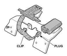
19. Using the two flange nuts attach the antenna bracket assembly to the dashboard support.
